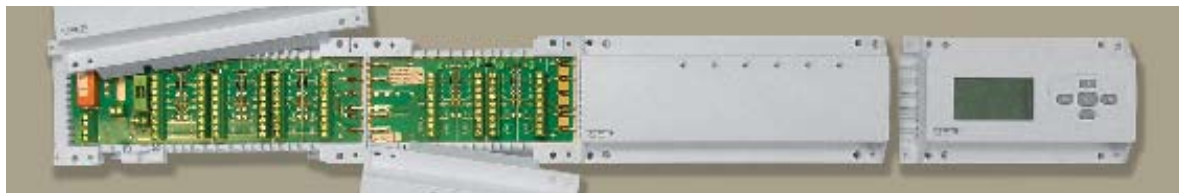
Zone Valve/Actuator assembly with outer covers removed to show the solid-state circuitry.
